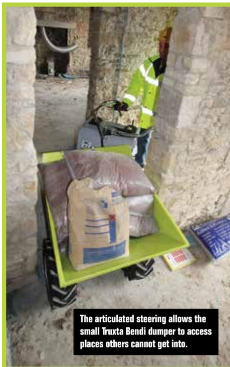
The articulated steering allows the small Truxta Bendi dumper to access places others cannot get into.
