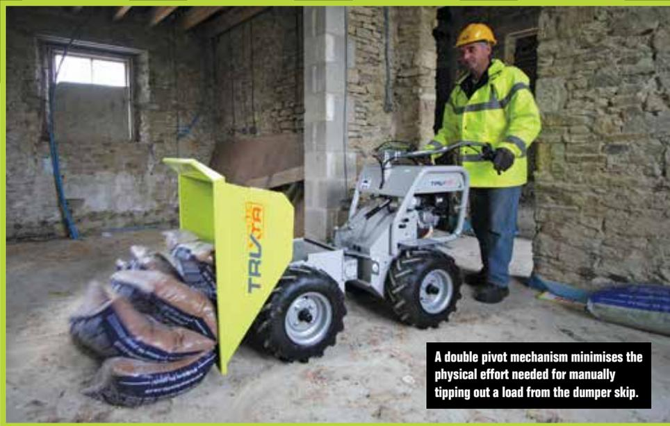
A double pivot mechanism minimises the physical effort needed for manually tipping out a load from the dumper skip.
