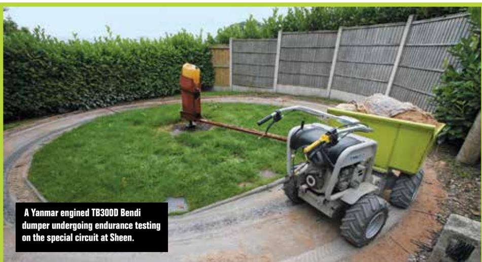
A Yanmar engined TB300D Bendi dumper undergoing endurance testing on the special circuit at Sheen.
