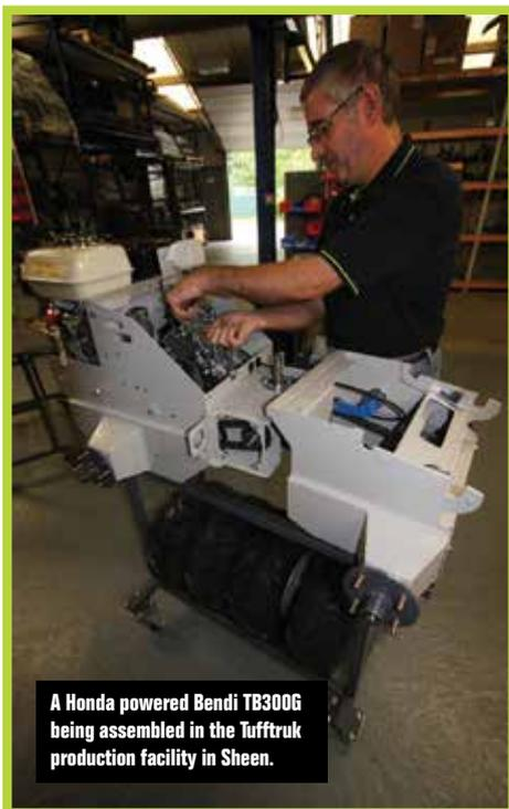
A Honda powered Bendi TB300G being assembled in the Tufftruk production facility in Sheen.
