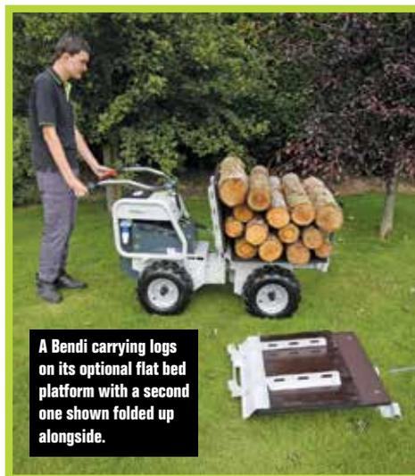
A Bendi carrying logs on its optional flat bed platform with a second one shown folded up alongside.
